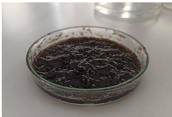
Fig.4. Chitosan-based graphene oxide (Ch@GO) hydrogel.
