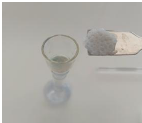
Fig. 3. Chitosan-based hydrogel for use in water purification
